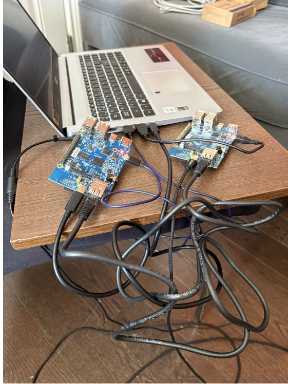
Figure 4: The Ethernet latency testing setup (side view).
