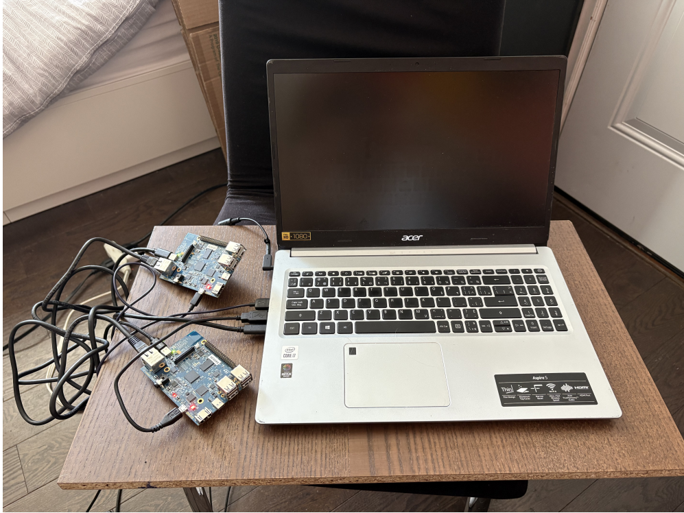
Figure 3: The Ethernet latency testing setup (front view).
